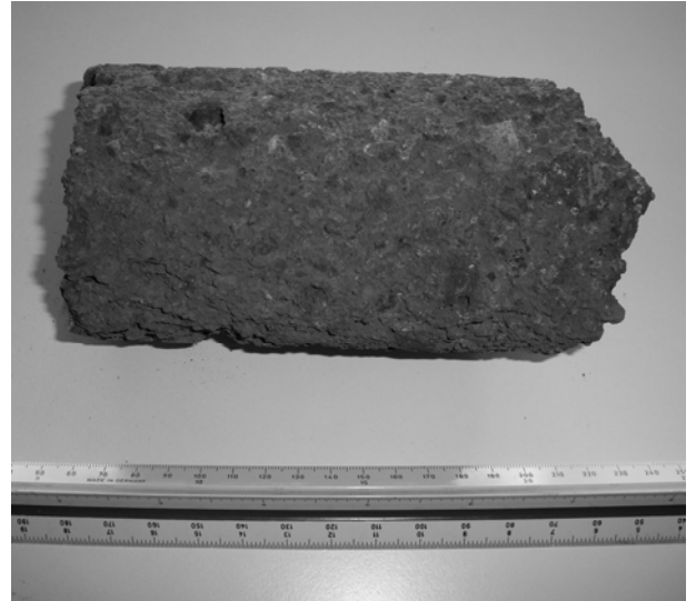
Figure 6: specimen of cemented pozzolana (PRb)
