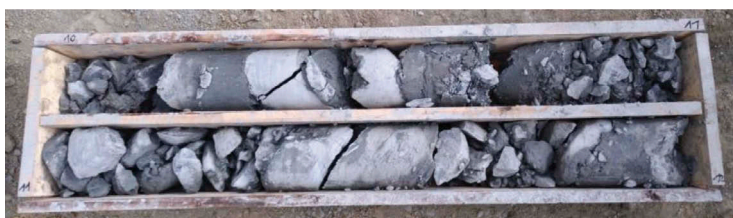
Figure 3. Hieroglyphic strata - typical borehole cores.
